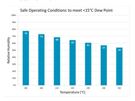
For safe operation of the Revio systems, the room must maintain a dew point of  $< 15^{\circ}$ C (59°F). Note that the peak air flow from the instrument is 2000 cubic feet per minute (CFM).
