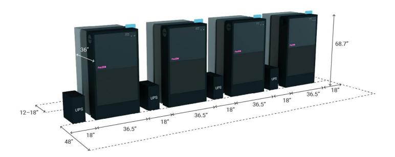
The general layout for multiple instruments is shown above. Note that up to 18" of open space is preferred behind the instrument, however, this can be reduced to 12" based on site-specific needs and limitations.
